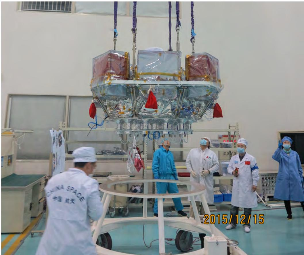
**Fig. 3** The payload assembly of HXMT in the process of integrating to the satellite
