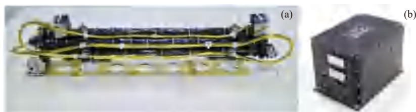
Fig. 12 FM of MAG boom (left) and electronic box (right)
