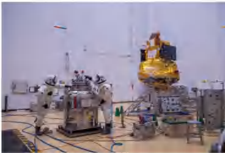
Fig. 19 SC was filled in propellant in S3 B
